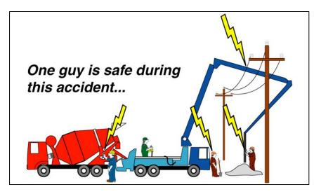
8. In the example below, a remote cable is touching the ground completing the path to the operator. Everyone involved in this accident is either injured or killed. The insulation of the remote cable is good for up to 600 volts, but the cable is energized to 8,000 volts. At that voltage, the insulation is ineffective, so the cable acts as a path to ground.
