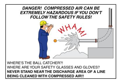
Never try to remove a blockage with compressed air. Remember, the pump can produce over 1,200 PSI on the material while an air compressor generates only 150 PSI. So, if the pump can't push it, air never will. The primary difference is that air is compressible while concrete is not; which creates the potential for a very dangerous release of energy.
