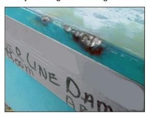
This next photo below proves wood conducts electricity. The outrigger pad was positioned on wooden cribbing when it struck the power line. You can see the hole left behind from the high voltage that traveled through the pad into the ground.
