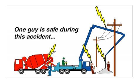
8. In the example below, a remote cable is touching the ground completing the path to the operator. Everyone involved in this accident is either injured or killed. The insulation of the remote cable is good for up to 600 volts, but the cable is energized to 8,000 volts. At that voltage, the insulation is ineffective, so the cable acts as a path to ground.
