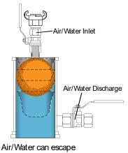
This blowout cap design has room between the air inlet and the discharge valve to allow the blowout ball or go devil to come back against the cap without blocking the air discharge. This will allow all residual air to be bled from the line before opening any clamps, potentially preventing explosion and injury.
