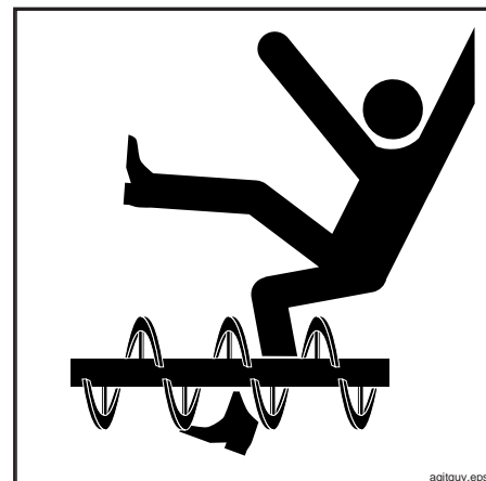
Figure 10 Lifting hopper grate exposes the agitator and the concrete valve
