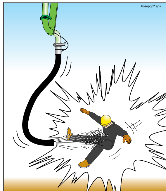
Figure 6 Remove everyone from the discharge area whenever the pump is first starting, restarting after moving, or if air has been introduced into the line
