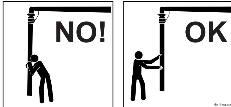
Figure 18 Do not hug the boom hose
