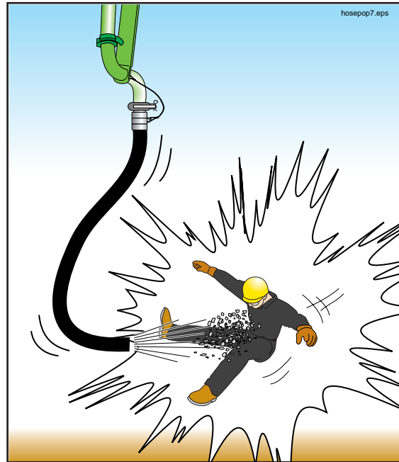
Figure 16 Stay away from the point of discharge when starting or restarting, and when there's air in the pipeline
