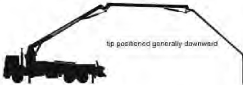
Figure 1, Position of Boom at Startup
