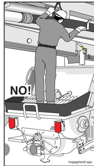
**4.13** There is only one operator of the concrete pump. The pump operator is responsible for the safe operation of the pump and boom. If you have questions regarding correct or safe pumping procedures, talk to the operator. Different operators may have different procedures, and this doesn't necessarily mean one of them is wrong. If in doubt, ask.
