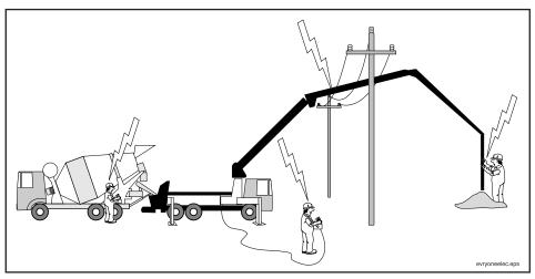
Figure 2 If the boom becomes energized, the mixer truck is also energized
