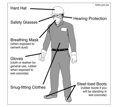
Figure 1 Wear the same protective clothing as the operator
