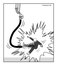
Figure 11 Release of trapped air is hazardous
