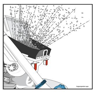
Figure 6 Concrete can splash from the hopper
