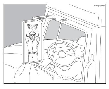
Figure 8 When backing, maintain visual contact at all times
