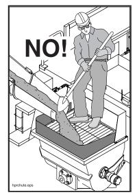
Figure 12 Stay out of the hopper **4.9 AWARNING! Projectile hazard.** Avoid walking under the boom of concrete pumping trucks. Avoid standing next to the elbow at the back of the pump.
