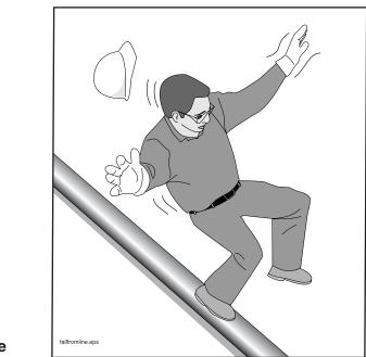
Figure 3 Never walk on the pipeline
